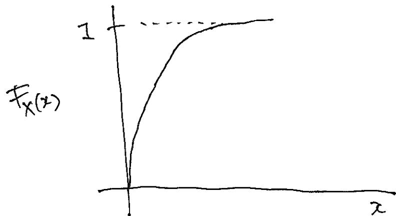
$$\begin{aligned} F_x(x) &= \int_0^x \frac{1}{\lambda} e^{-t/\lambda} dt \\ &= 1 - e^{-x/\lambda} \end{aligned} \quad x \geq 0$$
